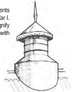
Woodworkers' Roof Ventilator Small - Height 980mm min. diameter - 200mm Base diameter 360mm Large - Height 1200mm min. diameter - 280mm Base diameter 500mm
